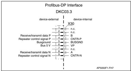
Fig. 4-184: Profibus-DP interface for DKC03.3
