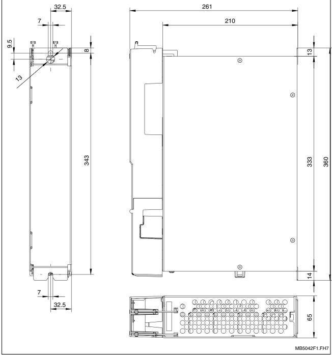
Fig. 7-1: Dimensions of the auxiliary capacitance module CZM01.3
