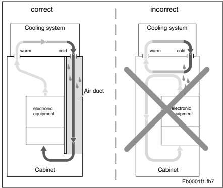
Fig. 12-19: Arranging cooling unit on cabinet
