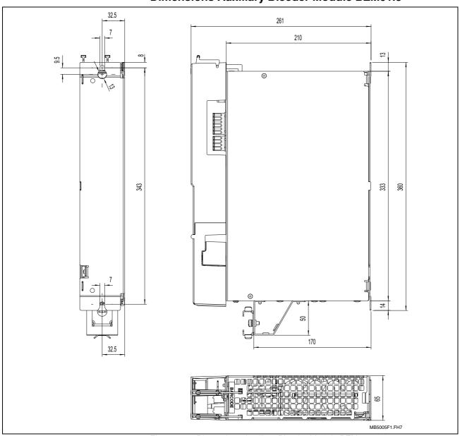
Fig. 6-1: Dimensions Auxiliary Bleeder Module BZM01.3
