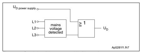
Fig. 4-148: Correlation of U<sub>D power supply</sub> and U<sub>D</sub> (U<sub>D message</sub>)
