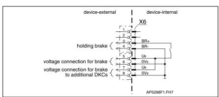
Fig. 4-103: Holding brake and voltage connection
