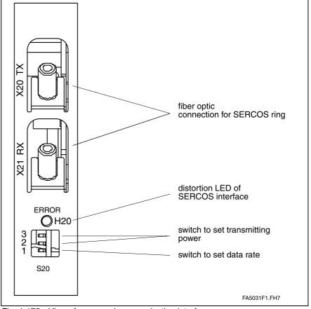
Fig. 4-175: View of command communication interface
