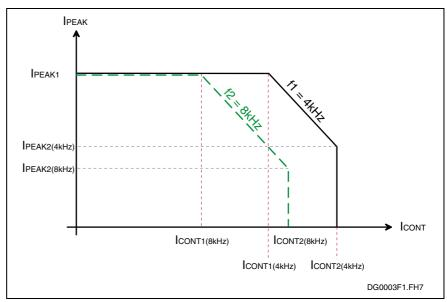
Fig. 4-16: Output current characteristic curves for servo applications
