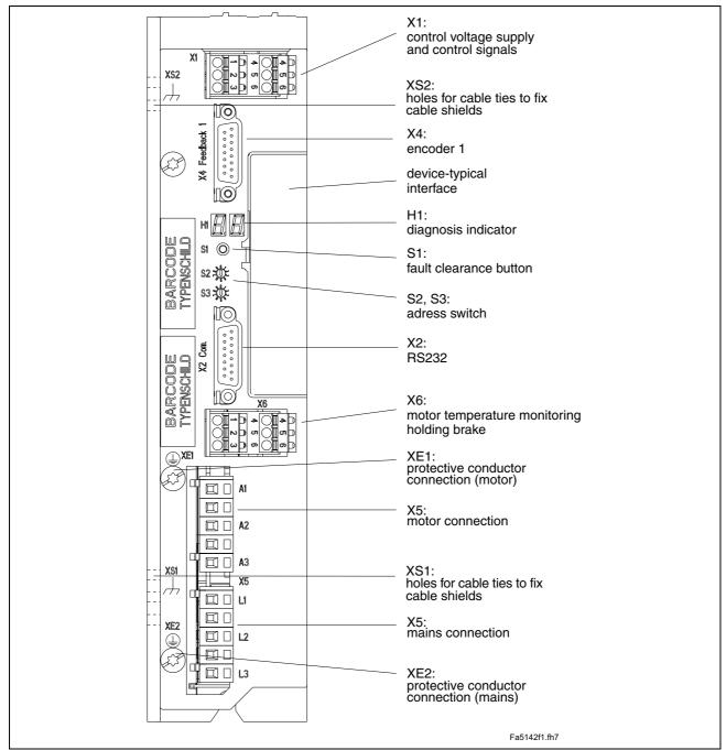
Fig. 5-19: Front view DKC\*\*.3-016 with connectors
