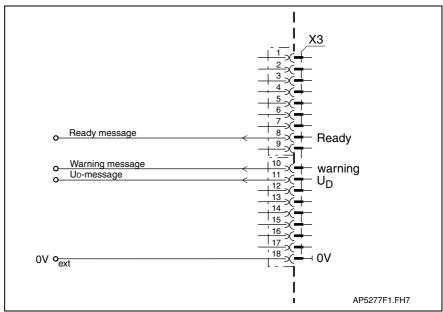
Fig. 4-69: Control outputs
