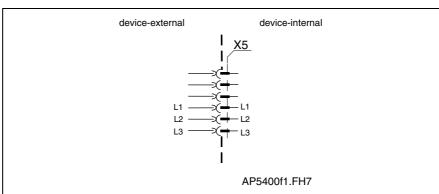
Fig. 5-58: Three-phase mains connection
