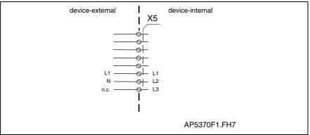
Fig. 4-96: Single-phase mains connection
