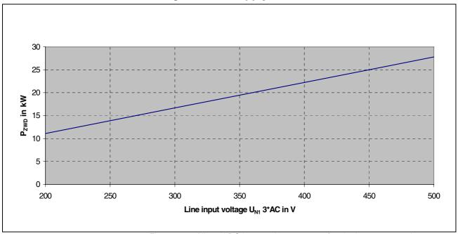
Fig. 4-35: Allowed DC bus continuous power for single source supply DKC\*\*.3-200-7 with CZM01.3 and filter choke GLD12
