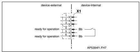
Fig. 5-29: Connections for ready to operate contact
