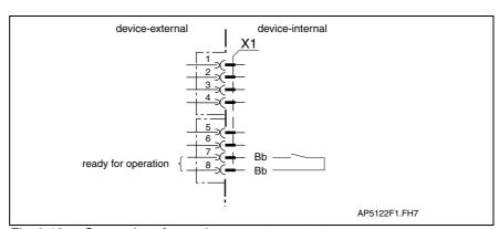
Fig. 6-16: Connections for ready to operate contact
