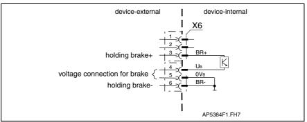
Fig. 5-64: Holding brake and voltage connection
