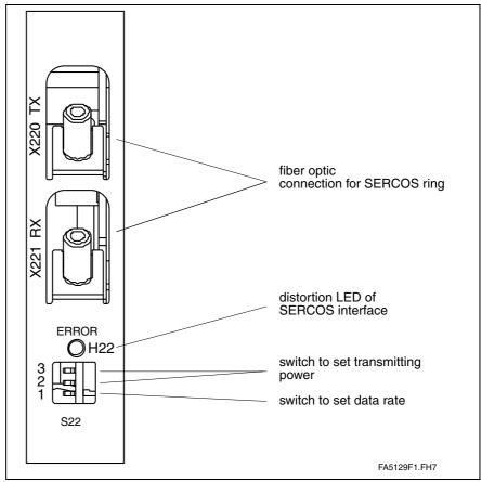
Fig. 4-220: View of command communication interface
