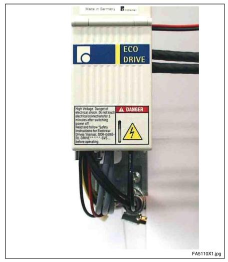
Fig. 16-28: View with contact protection
