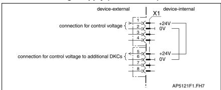
Fig. 4-51: Connections for control voltage
