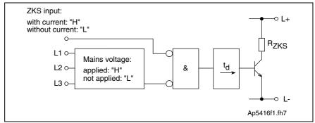
Fig. 6-25: Block diagram interlock ZKS/Mains
