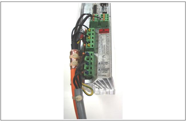
Fig. 16-27: Connection of motor and mains cable
