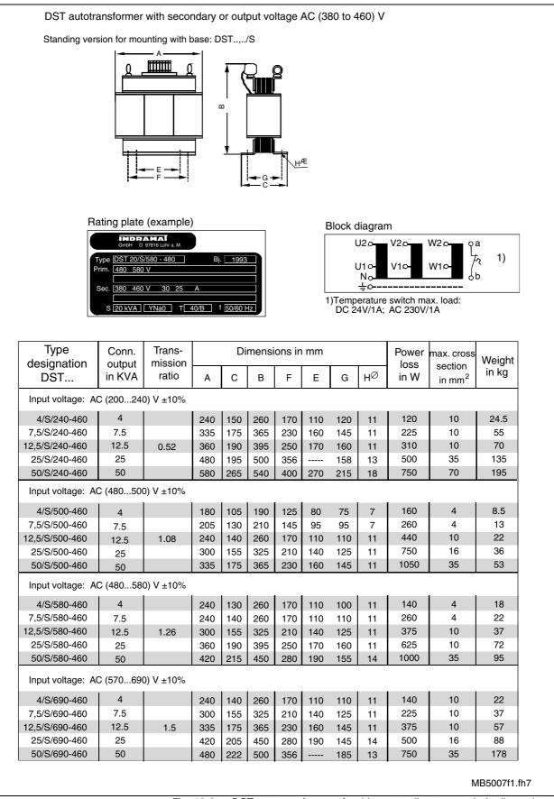
Fig. 10-2: DST autotransformers for drive controllers to match the line voltage
