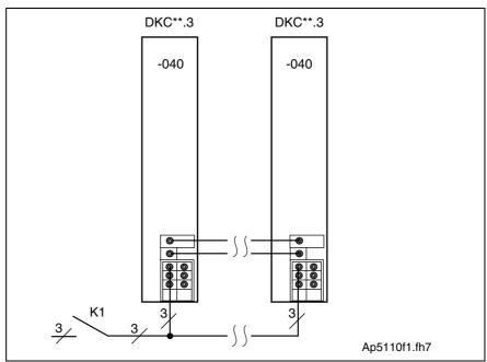
Fig. 4-24: Group supply with DC bus connection
