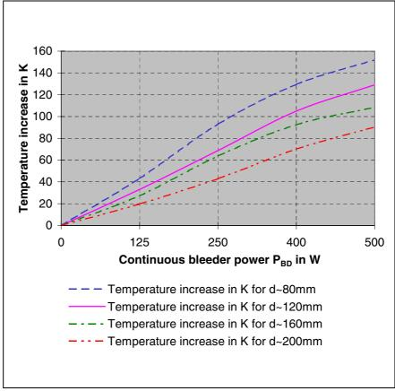
Fig. 12-13: Temperature increase DKC\*\*.3-100-7-FW
