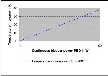
Fig. 12-11: Temperature increase DKC\*\*.3-016-7-FW
