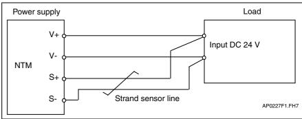
Fig. 9-6: Connecting the sensor cables NTM01.1-024-004 and NTM01.1-024-006
