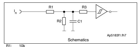
R2: 3k3 R3: 10k C1: no data Fig. 5-39: Input circuit
