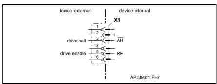
Fig. 5-26: Connections for drive halt and drive enable
