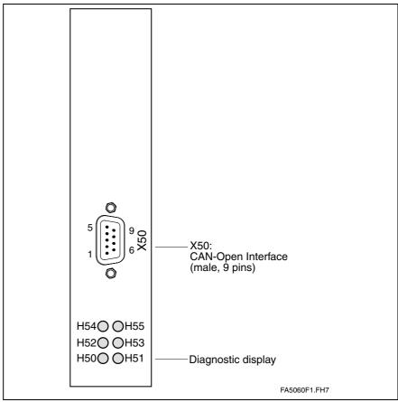
Fig. 4-199: View of command communication interface
