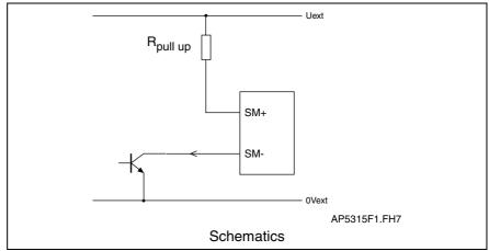
Fig. 4-173: Controlling with open collector outputs
