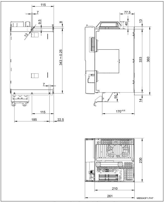
Fig. 4-3: Drive Controller DKC\*\*.3-200-7-FW
