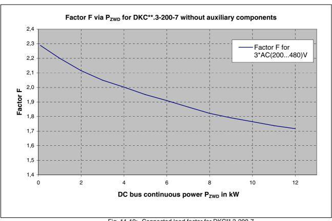
Fig. 11-10: Connected load factor for DKC\*\*.3-200-7
