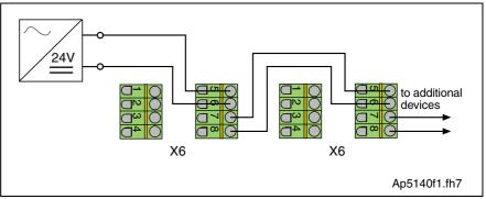
Fig. 4-105: Looping through the brake supply
