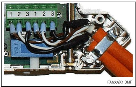
Fig. 16-36: Connecting the RS485 - Connectors
