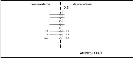
Fig. 6-41: Single-phase mains connection
