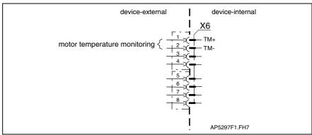
Fig. 4-101: Motor temperature monitoring
