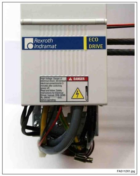
Fig. 16-30: View with contact protection
