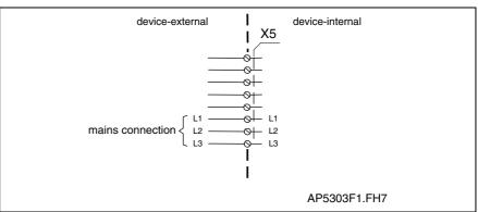
Fig. 4-97: Three-phase mains connection
