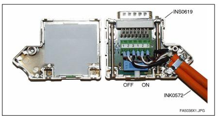
Fig. 16-35: Connecting the RS485 - Connectors
