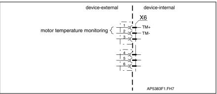
Fig. 5-62: Motor temperature monitoring
