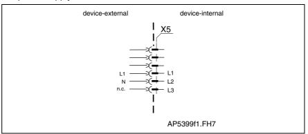
Fig. 5-57: Single-phase mains connection
