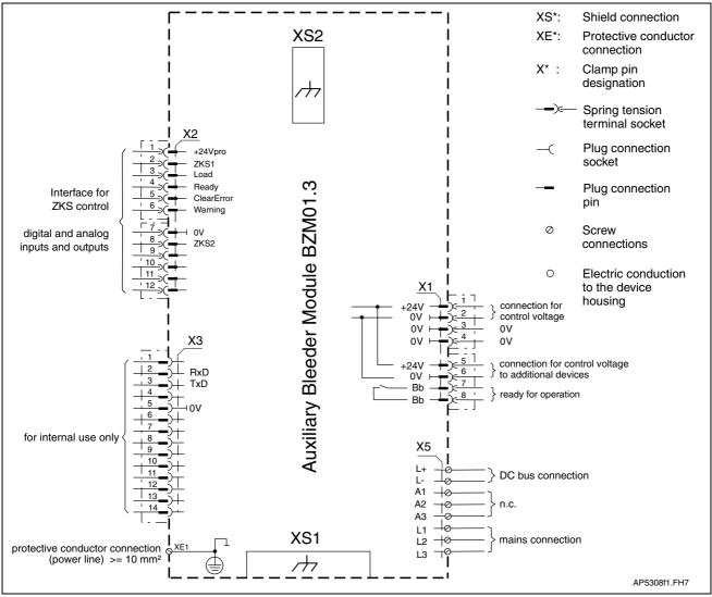
Fig. 6-9: Terminal diagram - BZM01.3
