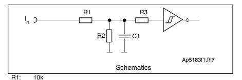
R2: 3k3 R3: 10k C1: no data Fig. 5-27: Input circuit
