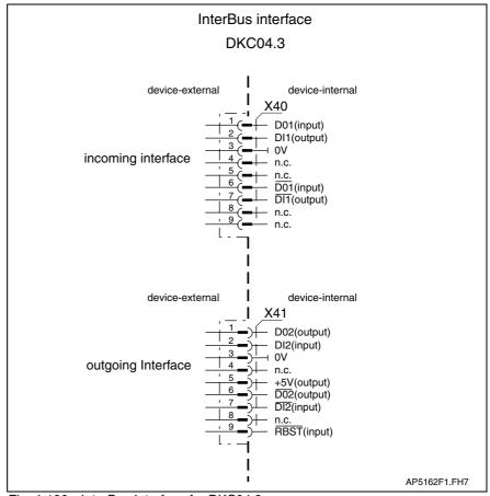
Fig. 4-196: InterBus Interface for DKC04.3
