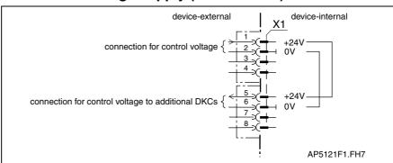
Fig. 6-14: Connections for control voltage
