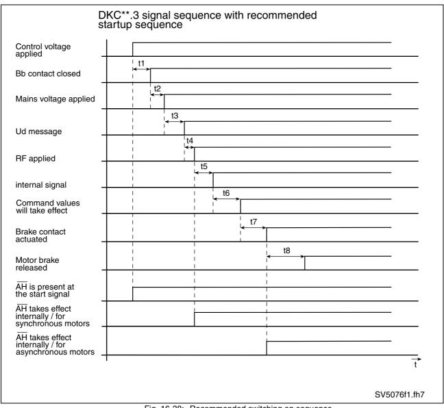
Fig. 16-38: Recommended switching on sequence
