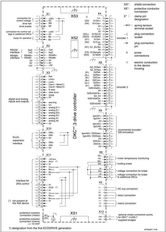
Fig. 4-47: Total connection diagram for DKC\*\*.3
