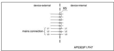
Fig. 6-42: Three-phase mains connection
