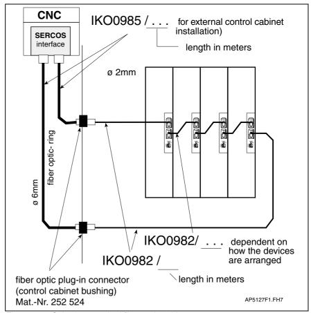
Fig. 4-180: Selecting standard fiber optic cables
