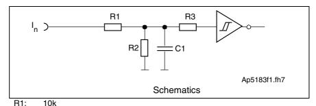
R2: 3k3 R3: 10k C1: no data Fig. 4-67: Input circuit
