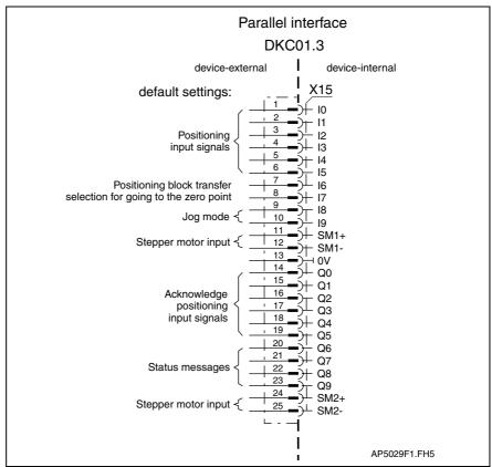
Fig. 4-162: Parallel interface for DKC01.3
