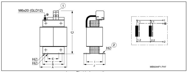
1: Electrical connection 2: Slot in "J" direction Fig. 8-1: Dimensions GLD 12
