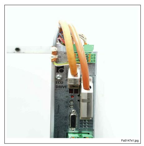
Fig. 16-19: View with Parallel Interface 2
