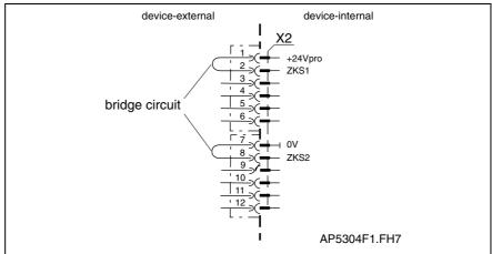
Fig. 6-20: Connection +24V pro, 0V
