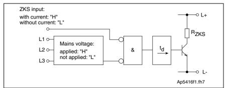
Fig. 4-146: Block diagram interlock ZKS/Mains
