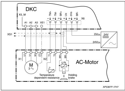
Fig. 5-66: Connection of motor cable, holding brake and temperature monitor for motors with connector box
