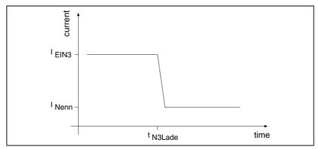
Fig. 5-6: Charging current profile of control voltage
