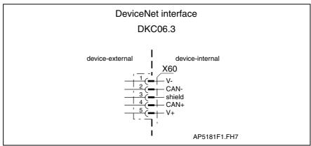
Fig. 4-207: DeviceNet Interface for DKC06.3
