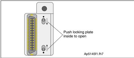
Fig. 15-4: Locking the programming module
