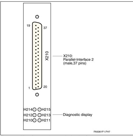
Fig. 4-210: View of command communications interface
