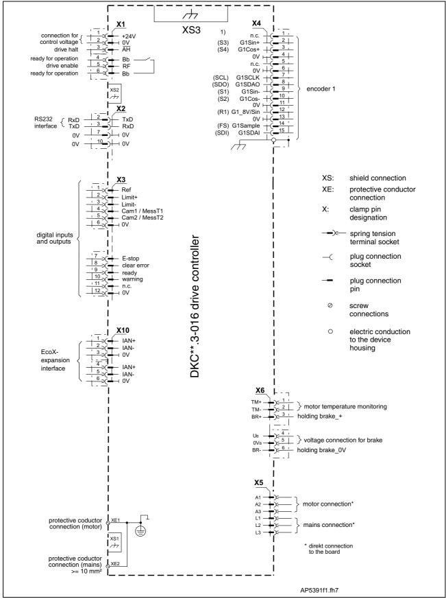
Fig. 5-21: Total connection diagram for DKC\*\*.3-016
