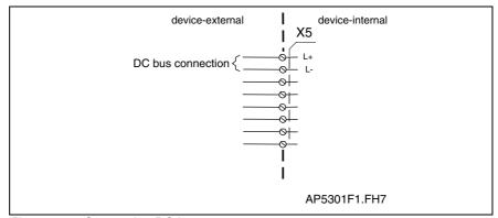
Fig. 6-39: Connection DC bus
