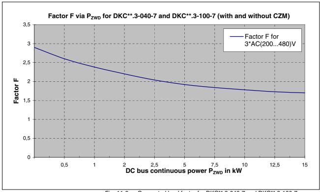
Fig. 11-9: Connected load factor for DKC\*\*.3-040-7 and DKC\*\*.3-100-7
