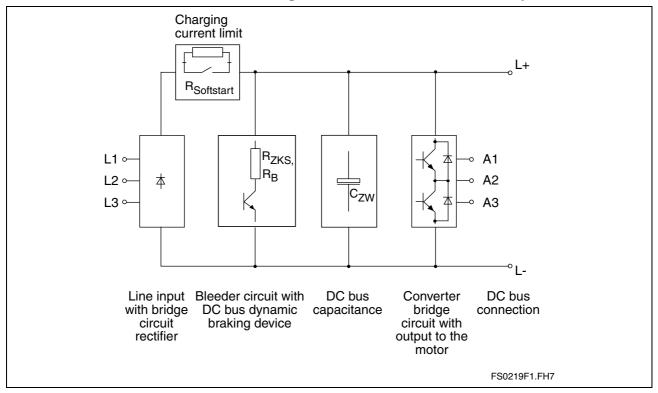
Fig. 4-9: Block diagram of the DKC\*\*.3-100-7-FW power section
