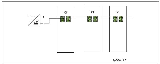
Fig. 16-11: Looping through the control voltage
