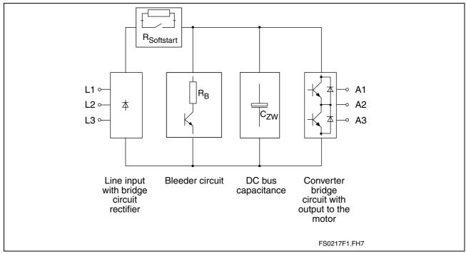
Fig. 5-4: Block diagram of the DKC\*\*.3-016-7-FW power section
