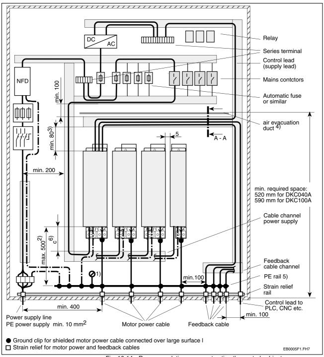
Fig. 16-14: Recommendations on constructing the control cabinet
