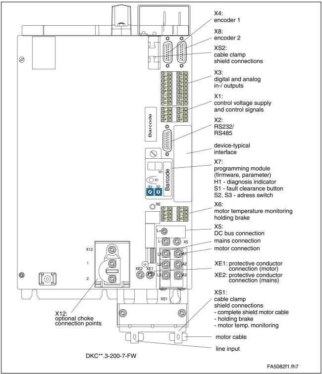
Fig. 4-44: Front view DKC\*\*.3-200-7-FW with connectors
