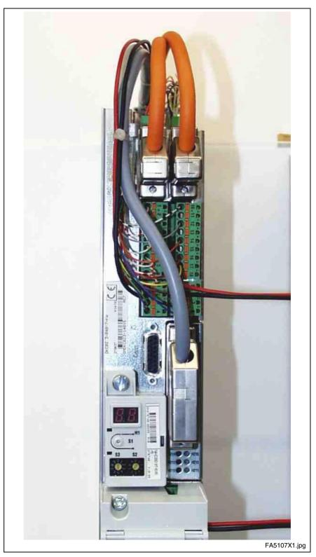
Fig. 16-24: View with Parallel Interface 2
