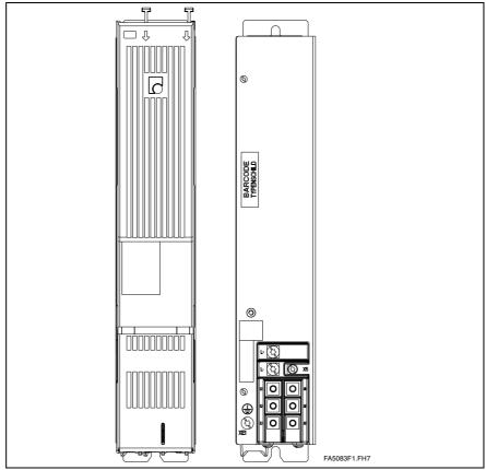
Fig. 7-7: Front view of auxiliary capacitance module CZM01.3
