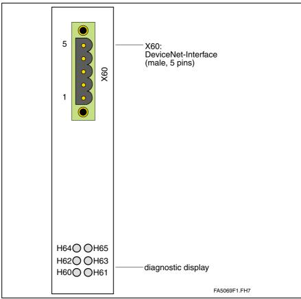
Fig. 4-204: View of command communication interface
