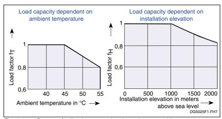
Fig. 4-4: Degree of utilization as a value dependent on ambient temperature and installation altitude
