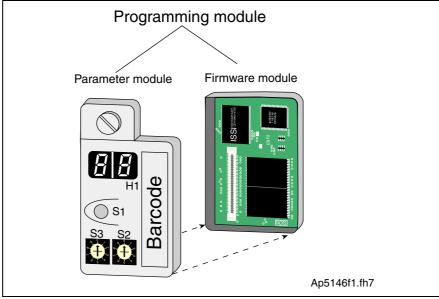
Fig. 4-108: X7, Programming module
