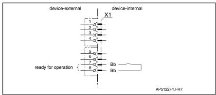
Fig. 4-56: Connections for ready to operate contact
