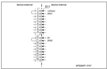
Fig. 4-141: DC bus dynamic brake control
