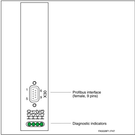
Fig. 4-181: View of command communication interface
