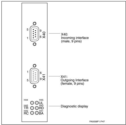
Fig. 4-193: View of command communication interface
