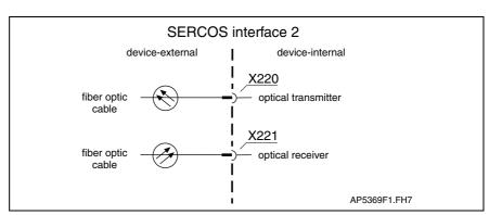
Fig. 4-221: I/O connection allocations
