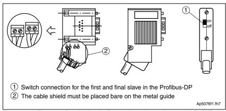
Fig. 4-191: Fig. 4-23: Bus link for the first and last slave without 9-pin D-SUB socket, INS 0540
