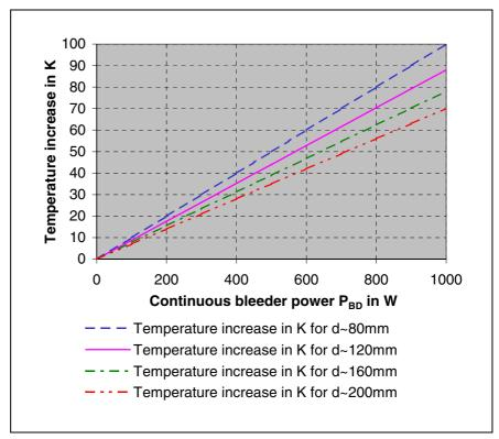
Fig. 12-14: Temperature increase DKC\*\*.3-200-7-FW
