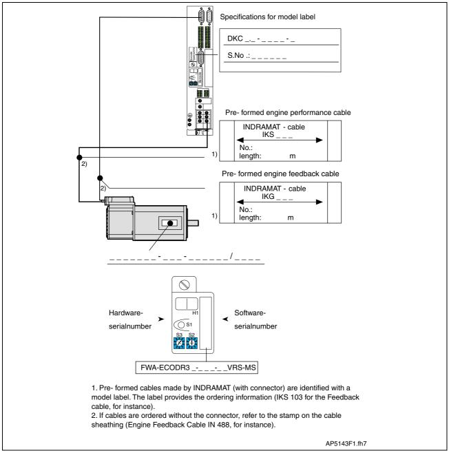
Fig. 15-1: Type designations of the drive components
