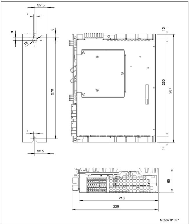
Fig. 5-1: Drive Controller DKC\*\*.3-016-7-FW
