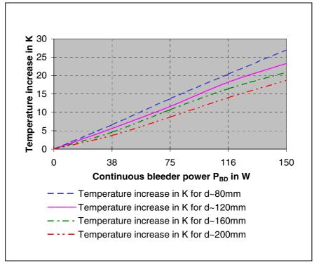
Fig. 12-12: Temperature increase DKC\*\*.3-040-7-FW
