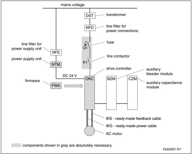
Fig. 1-2: Overview of individual components
