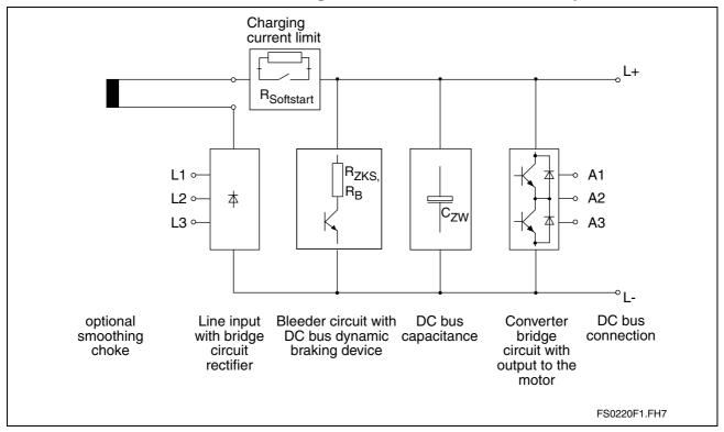
Fig. 4-10: Block diagram of the DKC\*\*.3-200-7-FW power section
