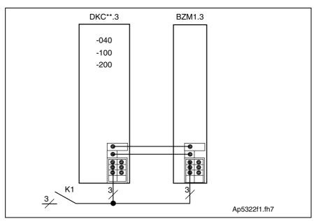
Fig. 6-10: DC bus and mains connection
