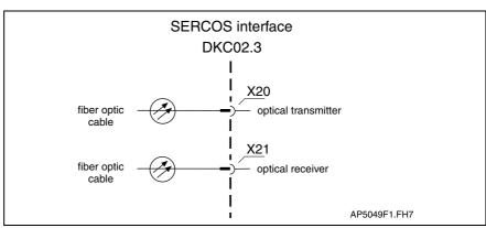
Fig. 4-176: I/O connection allocations for DKC02.3
