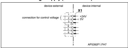
Fig. 5-25: Connections for control voltage
