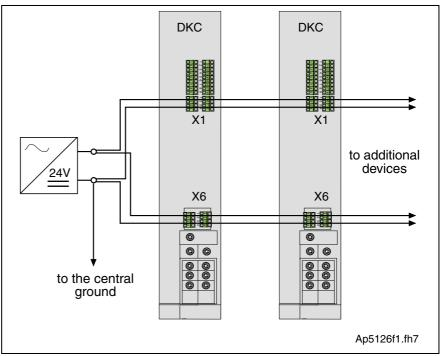
Fig. 4-104: Shared voltage source for brakes and control voltage supply
