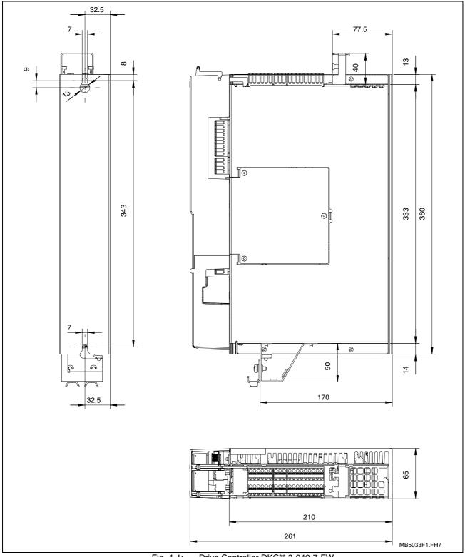
Fig. 4-1: Drive Controller DKC\*\*.3-040-7-FW
