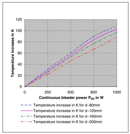
Fig. 12-15: Temperature increase BZM\*\*.3-01-7
