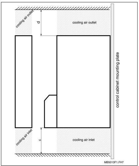
Fig. 12-10: Exit and entrance of cooling air
