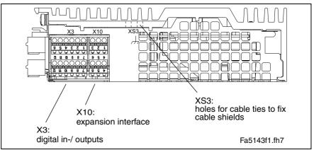
Fig. 5-20: Connections on top of unit for DKC\*\*.3-016-7-FW
