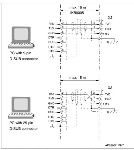
Connect the metallic connector case with the device potential using the fastening screws of the connector
