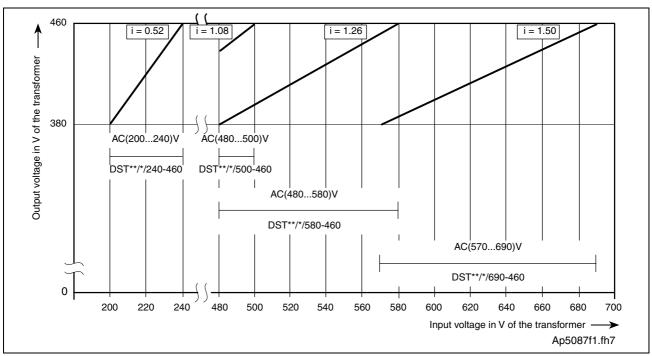
Fig. 10-1: Classification of three-phase autotransformers in rating groups
