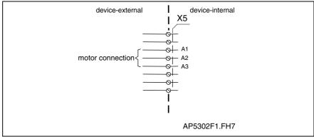
Fig. 4-94: Motor connections
