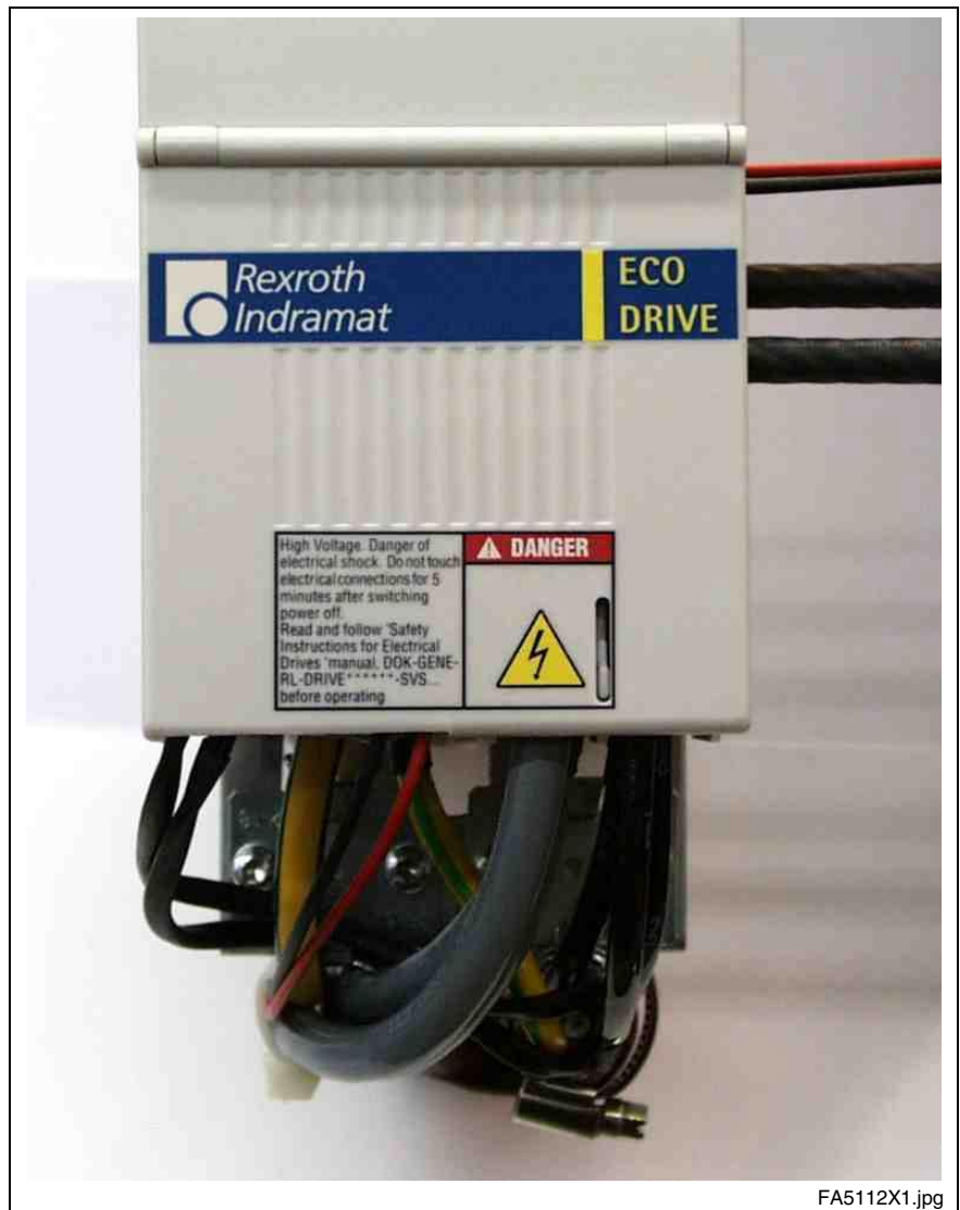
Fig. 16-30: View with contact protection
