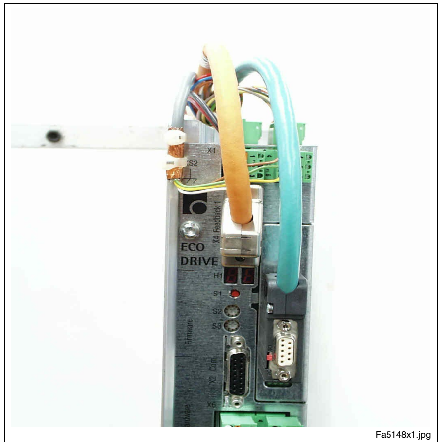
Fig. 16-18: View with Profibus-DP Interface
