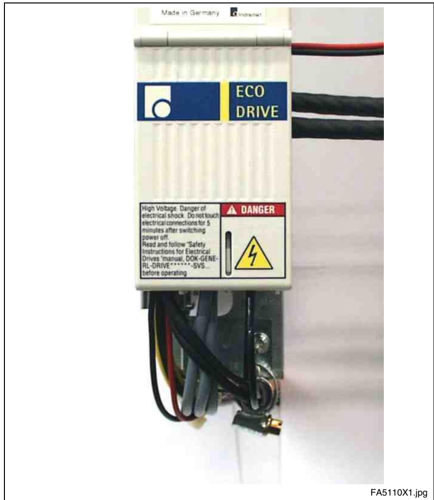
Fig. 16-28: View with contact protection
