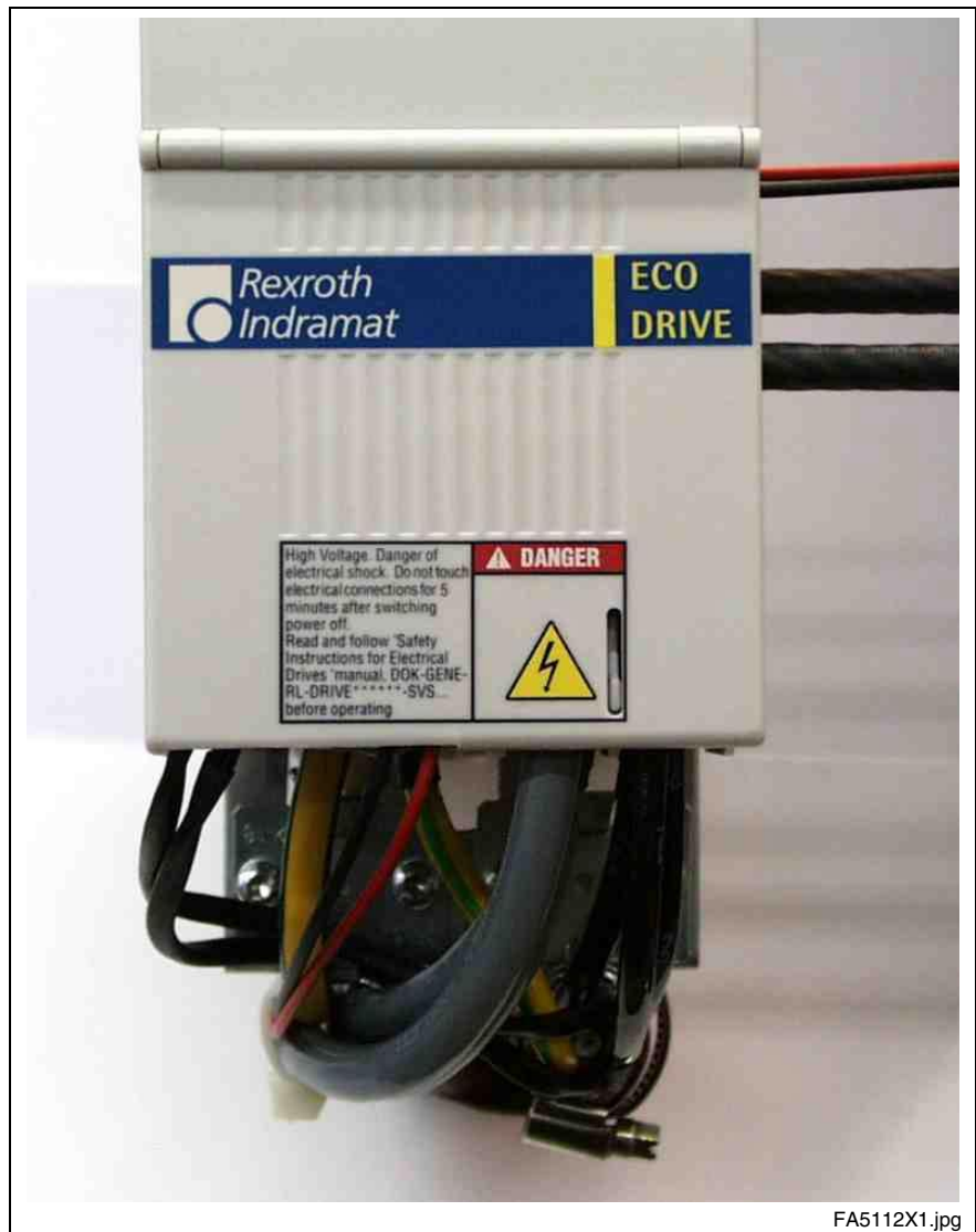
Fig. 16-30: View with contact protection
